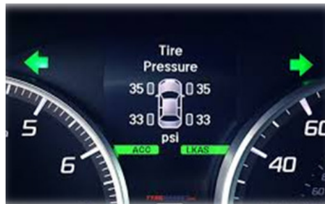
Fig 1.11: Tyre Pressure Monitoring System
