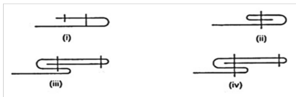
Fig (1.12): Hemmed edges (i) 504/103 (ii) 301 (iii) 2 \times 301 (iv) 2 \times 401
